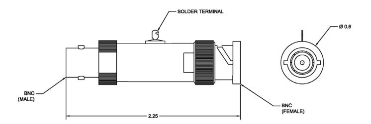
MPI's Model FTP-07 BIAS TAP is designed to solve the problem of introducing a DC voltage on an RF signal line while maintaining a well-disciplined 50 Ohm impedance.
